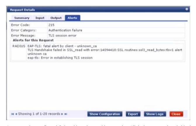
A customer has configured Onboard in a cluster with two nodes. All devices were onboarded in the network through node1 but those clients fail to authenticate through node2 with the error shown.
