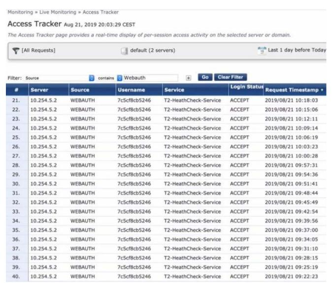
A customer has just configured a Posture Policy and the T 2 -Health check Service. Next they installed the OnGuard Agent on a test client connected to the Secure\_Employee SSID. When they check Access Tracker they see many WEBAUTH requests are being triggered.
