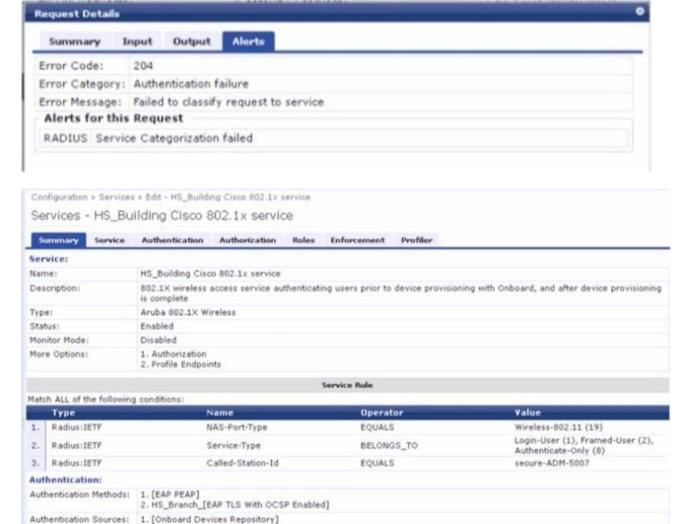
You configured a new Wireless 802.1 X service for a Cisco WLC broadcasting the secure-AOM-5007 SSID. The client fails to connect to the SSIO.
