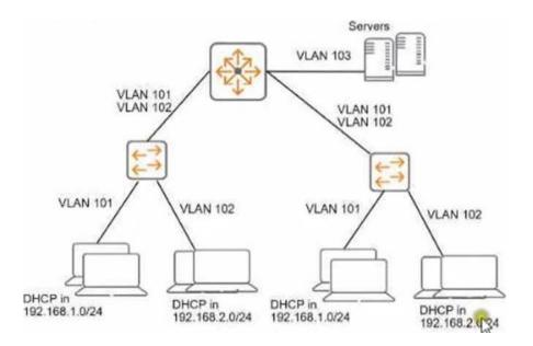
You need to ensure that only management stations in subnet 192.168.1.0/24 can access the ArubaOS-Switches' CLI. Web Ul. and REST interfaces. The company also wants to let managers use these stations to access other parts of the network.
